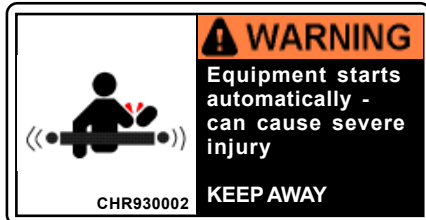
LOCATE AT ENTRANCE TO CONVEYOR WALKWAY
