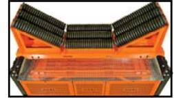
“Under high-volume conditions, standard OEM impact idlers in the load zone simply can't withstand heavy loads and lengthy drops, costing downtime for repairs as well as the expense of replacement components,” observed Martin Engineering Service Technician Doug Brown. The new cradles use Martin Engineering's Trac-mount™ technology to slide in and out easily for maintenance. The modular .....**Continue reading on Page 4**
