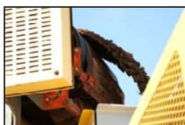
and durability as the model it replaces, while reducing the amount of urethane going to landfills. Manufactured with Martin Engineering's unique "CARP" (Constant Angle Radial Pressure) technology to maintain the most efficient cleaning angle throughout its service life, the Martin® QB1 Cleaner HD features a no-tool replacement process that can be performed safely by one person in less than five minutes. ....[Continue Reading](#)
