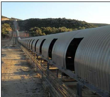
manufacturer, these new belt covers are described as rigid and strong. Characteristics include corrugated steel construction, a design that proves to be
