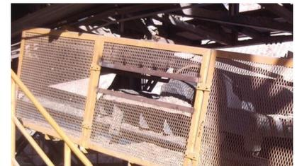
**Figure 1.** Inappropriate modification of guarding
