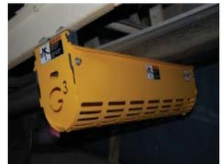
Appropriate labels should be used on the guards in order to help personnel identify the specific hazards associated with the guard. Labels may be custom made but may also be acquired from a variety of sources including CEMA. Signs may be employed if the affected area is large enough that a sign should be used in place of a label on or near the guard. Both labels and signs must be properly positioned, maintained and replaced as needed so that the hazard is identifiable by personnel.
